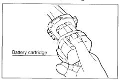
•Do not use force when inserting the battery cartridge. If the cartridge does not slide in easily, it is not being inserted correctly.
